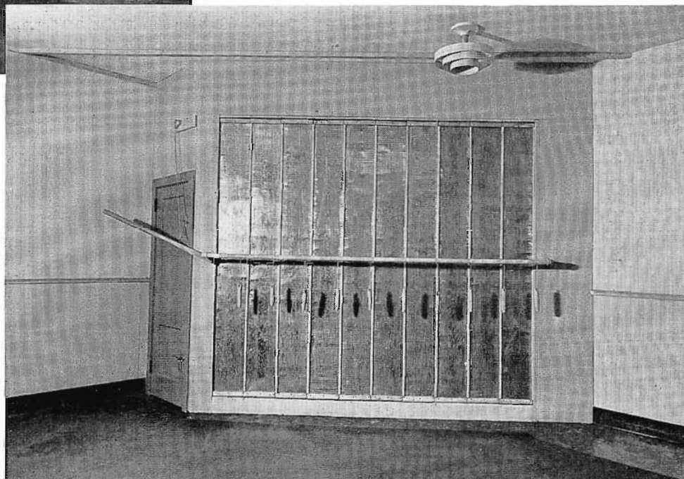
FIG. 5. (right) This view shows the vanes in the closed position (i.e. to cut off at approximately 5000 cycles as shown in Figure 6). Overlapping strips with felt gaskets, together with weights, insure a soundproof joint.
