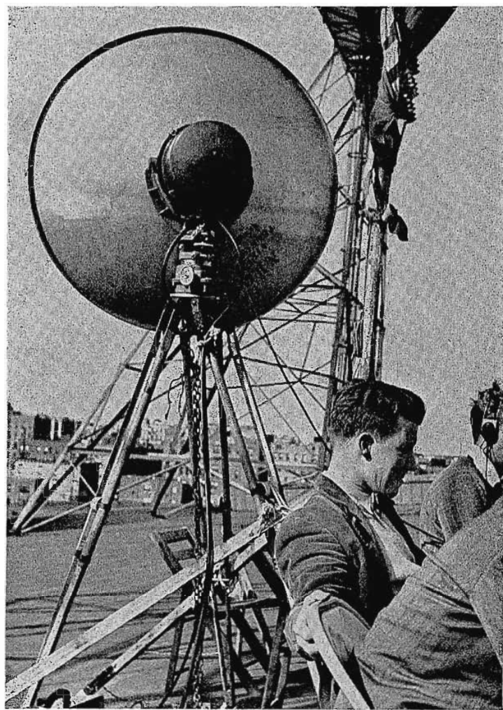
FIG. 5. Atop the grandstand at Ebbets Field, Brooklyn, the RCA Microwave transmitting parabola antenna lined up for a direct relay to the RCA Building.
